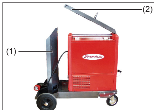
Removing the wirefeeder holder
